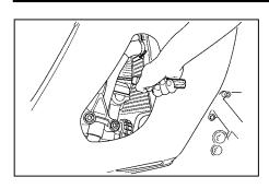
Check each spark plug for electrode erosion and excessive carbon or other deposits, and replace it if necessary.
