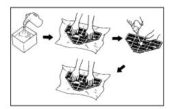
Apply oil of the recommended type to the entire surface of the sponge material, and then squeeze the excess oil out.
