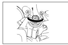
1. Spring preload adjusting bolt
