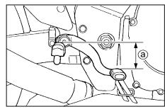
a. Distance between brake pedal and footrest
