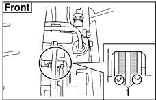
1. Front brake pad wear indicator ( $\times$  2)
