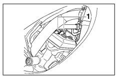
1. Spark plug cap (× 2 on each side)
