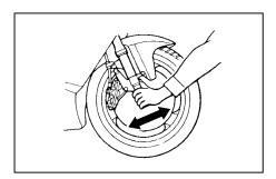
2. Hold the lower ends of the front fork legs and try to move them forward and backward. If any free play can be felt, have a Yamaha dealer check or repair the steering.
