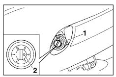
1. Compression damping force adjusting screw
